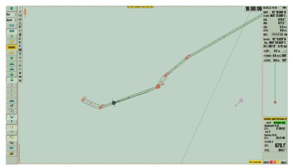
While this route monitoring view is selected, ETA waypoint texts are shown instead of Distance To Go (DTG). ETA times are also displayed with seconds as long as the time to go to the waypoint is under 24 hours.
