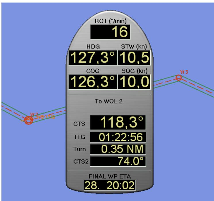
The mini conning has always been very useful for maneuvers and while anchored. Now we have improved on it, with the addition of a transit conning.
